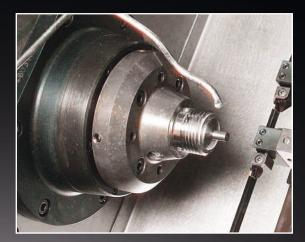
Finely adjustable pull-type and push-type clamping devices
