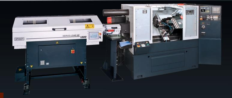
SPINNER SERVO short bar feeder for feeding bars up to a maximum of 1200mm
