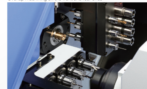
Overlap machining on the front and rear ends
